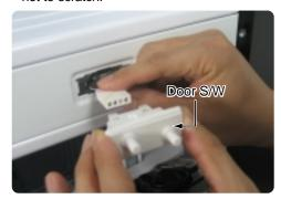
Disassemble the Cap Door S/W, Sleeve and the screws.
